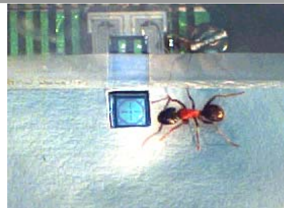
Figure 1: Carpenter ant C. vicinus with multi-axis force sensor
