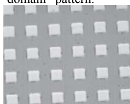
Figure 1: Optical image of array of 5 \mu\text{m} squares of CoZrTaTb spaced 5 \mu\text{m} apart.
