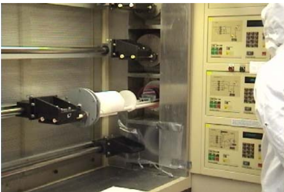
A silicon CVD deposition tool in SNF, with multiple furnace tubes
