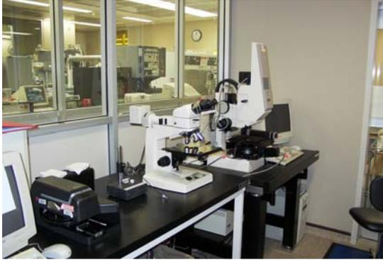
Characterization equipment in SNF, including microscopes and surface topography measurement tools
