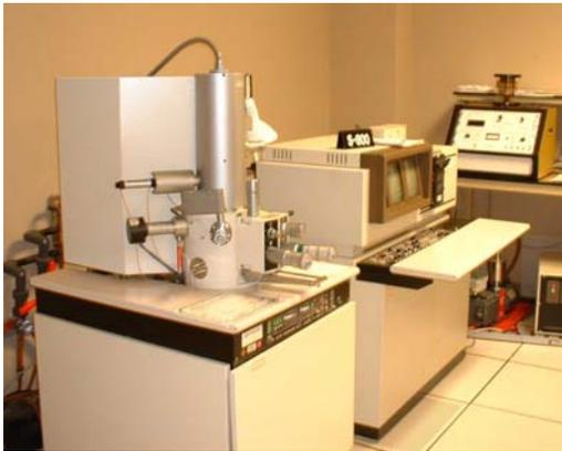
A scanning electron microscope (SEM) used to image nanoscale features
