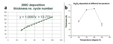
Fig. 3 a. Al2O3 deposited using standard recipe for 30 to 100 cycles. b. Al2O3 deposited for 100 cycles at 100C to 250 C.
