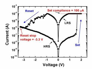
Fig. 1 I-V characteristics of HfO2/Al2O3 bi-layer RRAM devices. The device can set from high resistance state (HRS) to low resistance state (LRS) by a positive voltage sweep, and reset from LRS to HRS by a negative voltage sweep.
