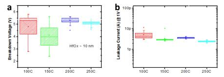
Fig. 9 a Breakdown voltage of HfOx deposited at 100C to 250 C to similar thickness ( $10\pm0.5$ nm). b Leakage current of HfOx deposited at 100C to 250 C to similar thickness ( $10\pm0.5$ nm).
