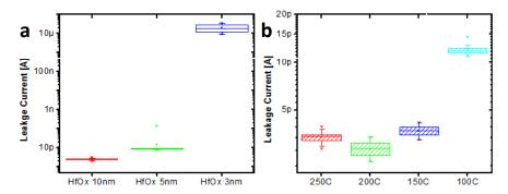
Fig. 8 a. Leakage current of HfOx deposited using standard recipe for 30 to 100 cycles. b. Leakage current of HfOx deposited for 100 cycles at 100C to 250 C.
