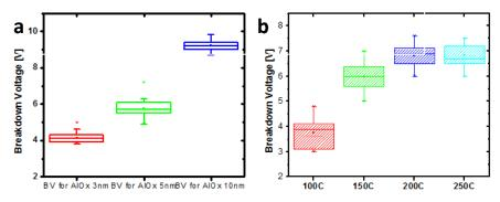
Fig. 5 a. Breakdown voltage of Al2O3 deposited using standard recipe for 30 to 100 cycles. b. Breakdown voltage of Al2O3 deposited for 100 cycles at 100C to 250 C.
