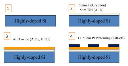
Fig. 2 Process flow for the MIM device structure
