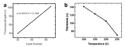
Fig. 4 a. HfOx deposited using standard recipe for 30 to 100 cycles. b. HfOx deposited for 100 cycles at 100C to 250 C.
