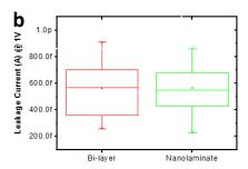
Fig. 10 a. Breakdown voltage of bi-layer oxide and nanolaminate oxide. b Leakage current of bi-layer oxide and nanolaminate oxide.
