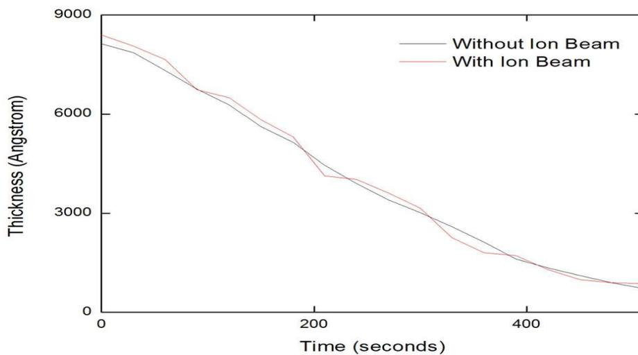
Figure 5: Etching over time of the sputtered SiO<sub>2</sub> films
