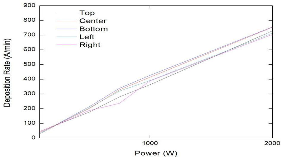
Figure 2: Titanium deposition rates on a 4-inch silicon wafer
