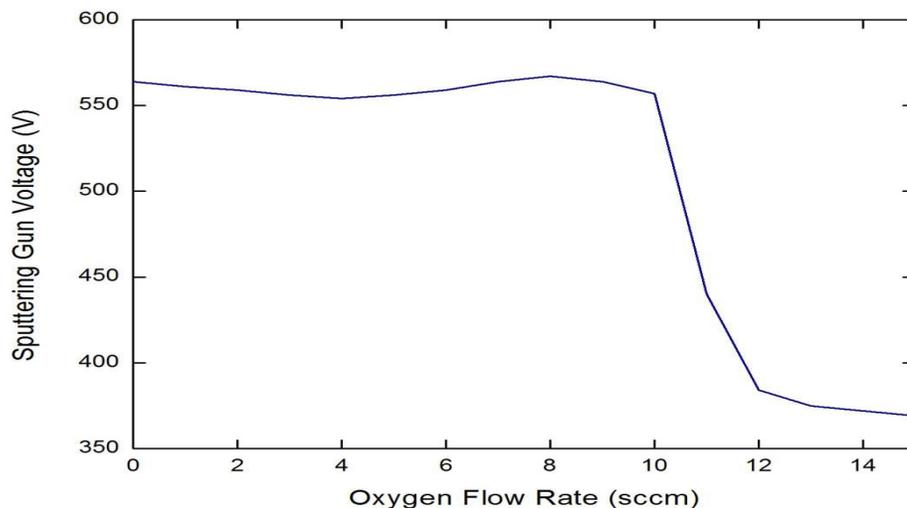
Figure 3: Sputtering gun voltage as a function of the O<sub>2</sub> flow rate
